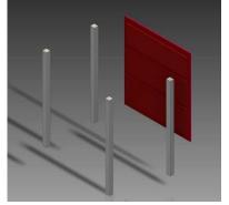
Place three of the four corner posts into the base. Do not glue if you want to remove the base later.
