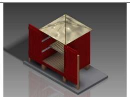
Attach the last corner post then the remaining side. Install the ceiling then the roof. Laminate the doors. Place the door stop posts in the base. Attach the doors.
