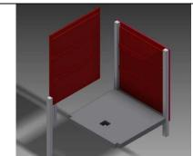
Attach one side wall and the lower floor support.
